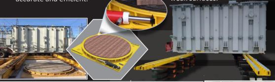
Our Jack & Slide System is used to relocate items up to 500tons. It makes use of vertical hydraulic jacks and the turn table to move items such as heavy transformers into its final position. This system is ideal for use in areas with space and height limitations where vehicles can not access.
